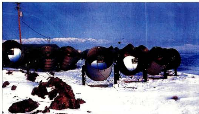
The Utah Fly's Eye detector (1981–1993) provided milestone cosmic ray measurements.
