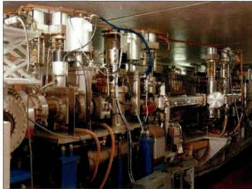
Part of the ALS storage ring at the Lawrence Berkeley National Laboratory. Frequency mapping was first applied to measured rather than simulated electron trajectories at the ALS.
