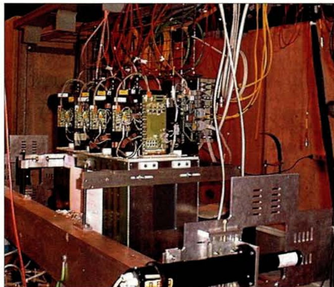
Fig. 2. A small-scale prototype set-up of the CMS experiment's tracker analogue read-out, timing distribution and on-detector slow-controls system under evaluation in CERN's 25 ns structured test beam.
